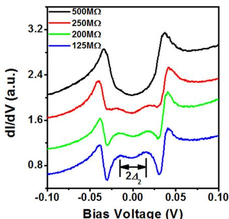
FIG. 3.  $dI/dV$  curves taken at different tunneling resistance of tunneling junction formed between STM tip and surface. The curves are shifted vertically for clarity.
