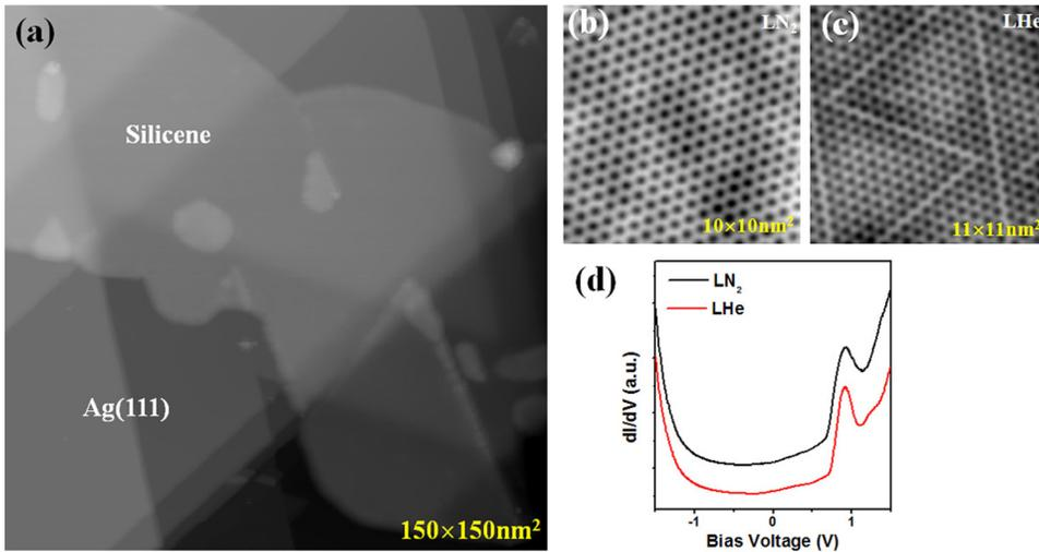
FIG. 1. (a) STM image of a monolayer silicene film on Ag(111) substrate, running across several Ag(111) steps. (b) and (c) High resolution STM images of silicene taken at tip bias 1.0 V at 77 K and 5 K, respectively. (d)  $dI/dV$  curves taken at 77 K (black curve) and 5 K (red curve), showing overall similar behavior (except the zero-bias gap which is too small to show in this voltage range). The curves are vertically shifted for clarity.
