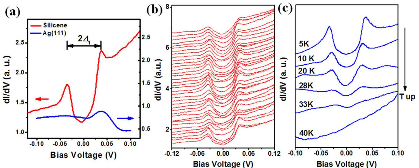
FIG. 2. (a)  $dI/dV$  curves obtained on silicene (red curve) and Ag(111) substrate (blue curve), respectively. (b) A series of  $dI/dV$  curves taken along a 15 nm line on silicene film, illustrating the uniformity of the gap. (c) Temperature dependence of  $dI/dV$  curve at same silicene film. The curves in (b) and (c) are shifted vertically for clarity.
