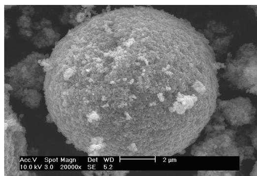
Fig. 2. The SEM image of the as-prepared  $\text{Li}_4\text{Ti}_5\text{O}_{12}$ .
