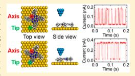
indicates that the mechanism of modifying the rotational potential is a combination of the van der Waals interaction and the interaction between the molecular dipole and an electric field. This work provides insight into the methods used to modify the effective rotational potential energy of molecular rotors.
