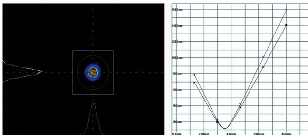
Fig. 4. (Color online) Far-field beam profile and  $M^2$  factor of the NOPA signal after subsequent multipass amplification in the second CPA stage as measured by a commercial beam analyzer (Spiricon  $M^2$ , 200 s).
