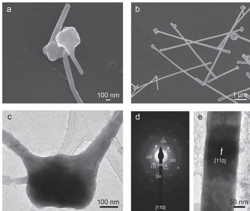
**Figure 2.** (a) SEM image showing copper nanorods sprouting from spherical copper seeds at a reaction time of 3.5 minutes. (b) By 20 minutes the rods had grown to form longer wires. (c) TEM image of two CuNWs growing out of a nanoparticle. (d) A selected area electron diffraction pattern (SAED) from the nanowire shown in (e) indicates the nanowire grew along the  $[1\bar{1}1]$  direction.
