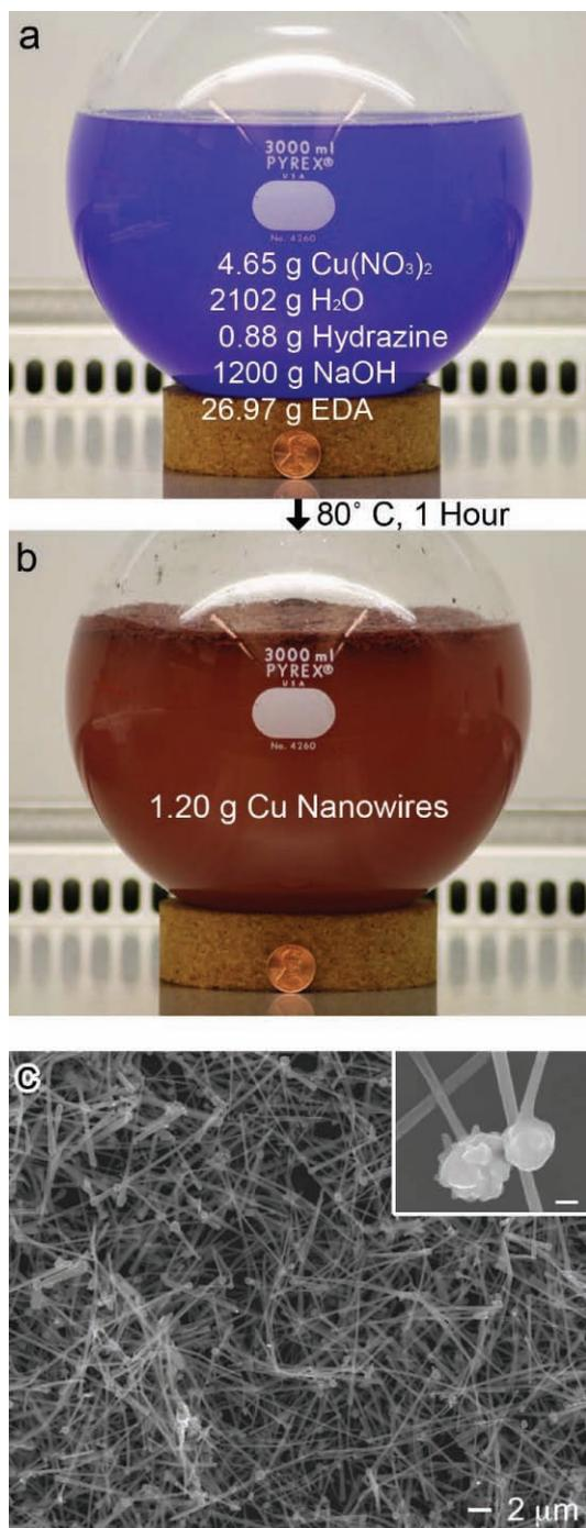
**Figure 1.** Pictures of the reaction flask (a) before the synthesis and (b) after growth of CuNWs at 80 °C for 1 hr. (c) SEM image of CuNW product. The nanowires are  $90 \pm 10$  nm in diameter and  $10 \pm 3$   $\mu$ m in length. The inset shows CuNWs with a spherical copper particles attached at one end (scale bar = 200 nm).
